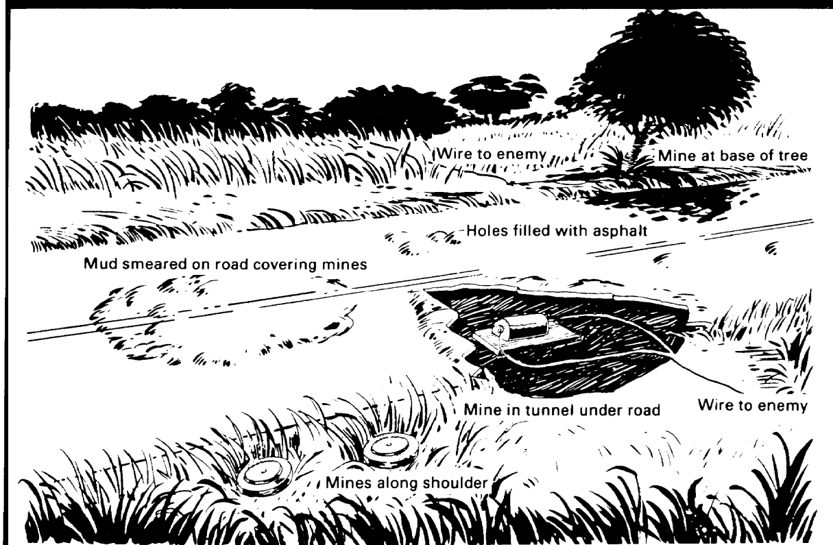
FIGURE 4-2. MINED HARD-SURFACE ROAD
